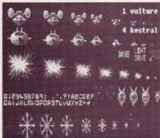
● Figure 1. This is how we did 3D Starfighter . Obviously the more steps you use the smoother the flow of the game - but equally obviously more steps means more memory eaten up
