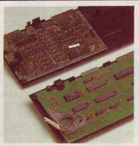
● Top: the new, lighter design: difficult to fix. Below, the old roomy circuit board
