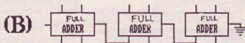
● Figure 5(B): how binary numbers of much larger than one can be added together
