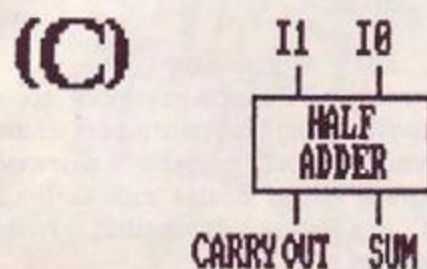
● And figure 4(C): any larger device – a calculator, for instance – would refrain from too much detail, and simply draw a symbol like this
