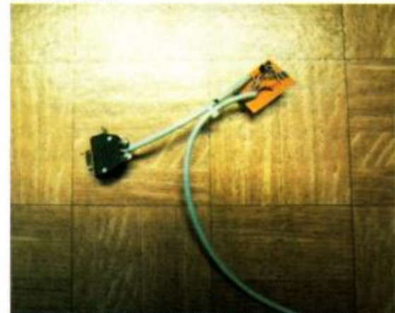
● The prototype lead in all its naked glory. Production versions will have the circuitry moulded into the joystick D-connector.
