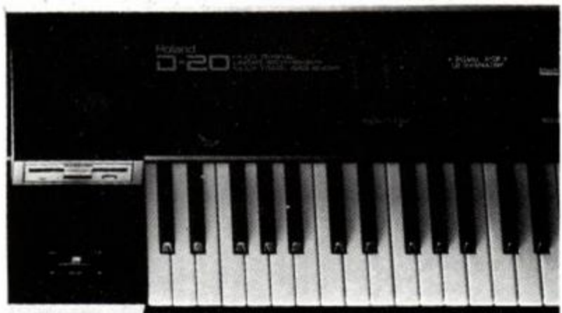
● Roland D-20: 3.5-inch disk drive and 9-track sequencer built-in.
