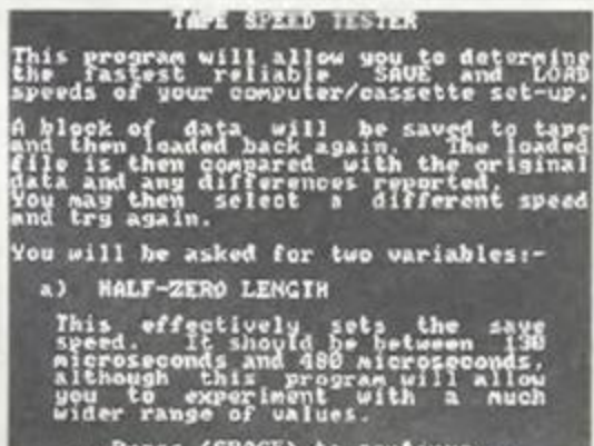
Tapetest lets you vary the baud rate of your tape unit to find the highest speed at which you can transfer data.
